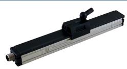
The working principle of ILT-110series inductive linear position sensors depends on the RLC coupling between the positioning element and the sensor. An output signal is provided according to the position of the positioning element. Thanks to the touchless working principle, they are long-lastingsince there are no factors such as wear and tear.
